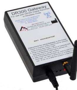
The Gateway is a transceiver (transmitter + receiver) that communicates with the wireless recorder. The Gateway sends the encrypted data via a wireless phone network to the receiving location. Both the recorder and the Gateway are able to transmit
