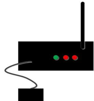
times in a row, there is a questionable connection with the cellular network, and the Gateway should be moved to a better connection. If the light only does a single blink, there is no connection at all to the wireless network.
