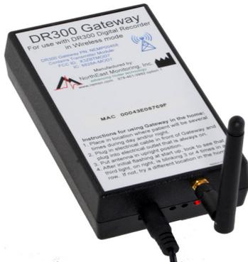
1. The Gateway should be placed in a location that the patient will be near (within 10 meters) frequently.
